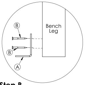
**Step B**Screw 1-5/8" screws (B) into bench leg.
