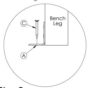
**Step C**Screw 2" screws (C) into mounting surface.
